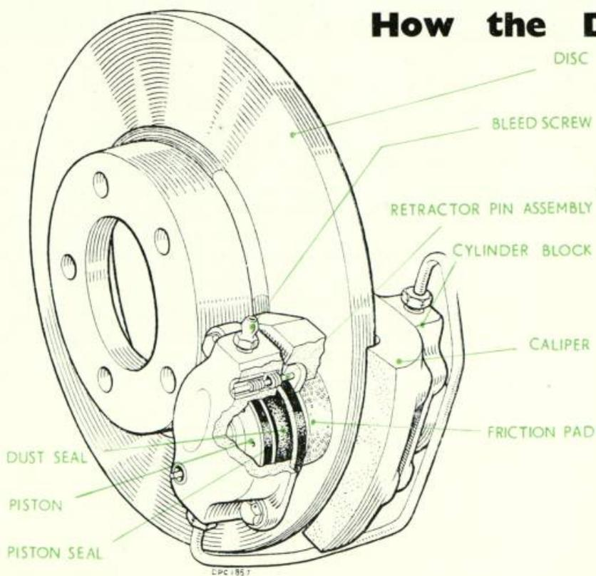
The illustrations on these pages clearly show the construction and operation of a Dunlop disc brake.
