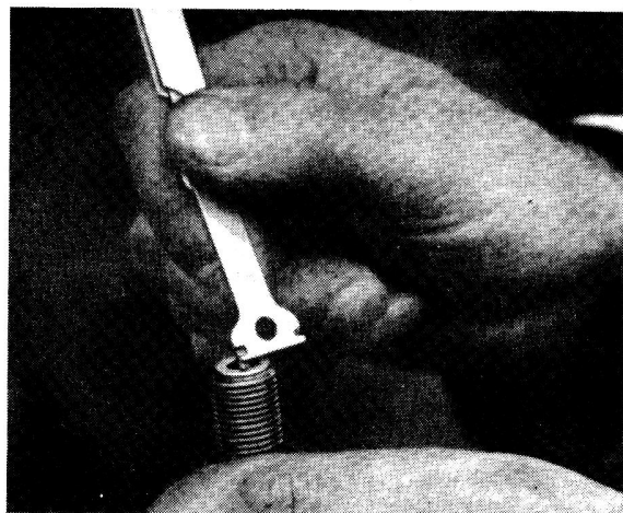
Fig.4.7. Setting the plug gap
