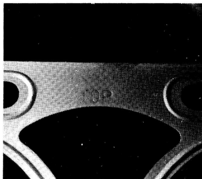
72.3b. Marking on cylinder head gasket
