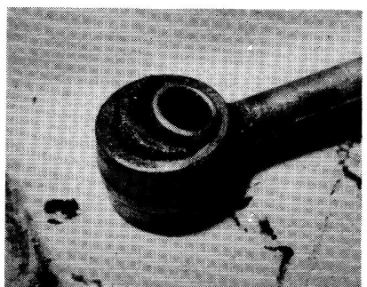
47.1. Engine stabiliser - perished rubber
