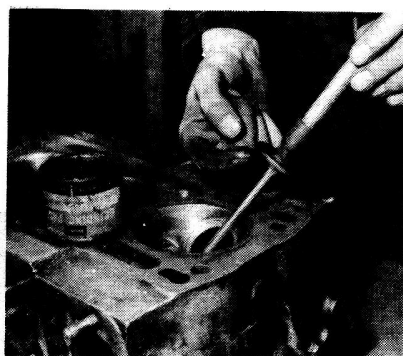
37.5b. Smear of carborundum paste on valve
