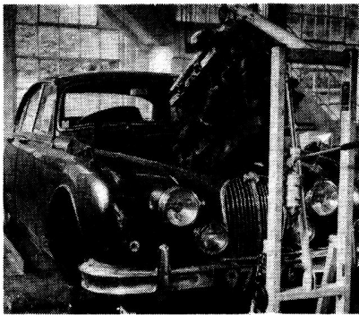
5.62. Lifting engine - stage 4
