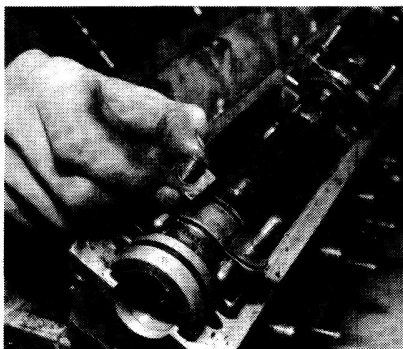
15.2. Camshaft bearing cap 'D' washer
