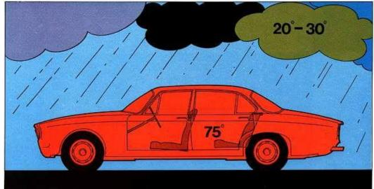
In this condition the automatic air conditioning system would select full heating to bring temperature up to chosen level.
