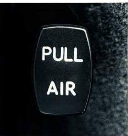
Whichever operating mode the heating system is set at, the rear passengers have a central multi-directional vent with an "OFF" position. They also have individual "volume" controls for left and right hand rear footwell supply. With or without the main system switched on, the driver and front passenger have an ON/OFF control for a separate supply of fresh air to the footwells, air for which is channelled from intakes above the outer headlamps.
