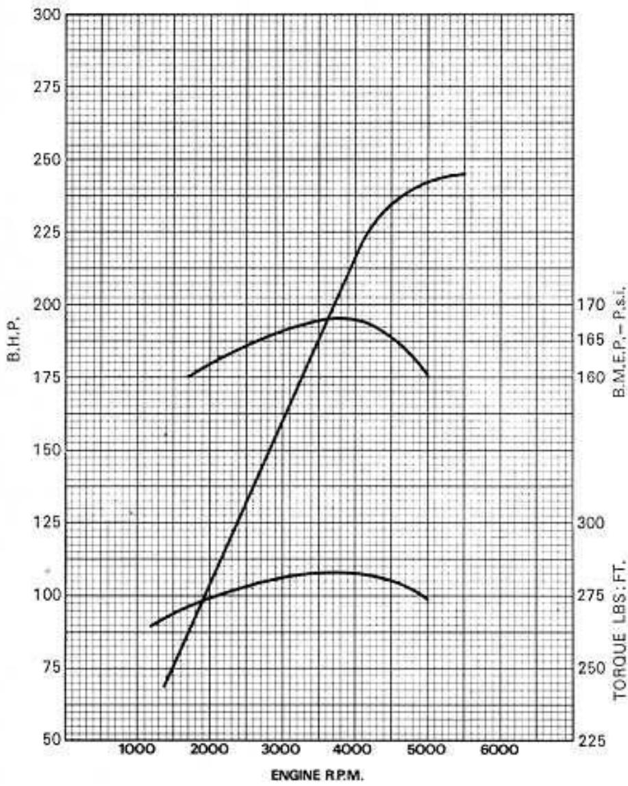
**ENGINE - 4.2 LITRE** In-line six cylinder, twin overhead camshaft engine with straight port type cylinder head. Twin S.U. H.D.8 carburetters, automatic enrichment control, and dual exhaust system. 92.07 mm bore x 106 mm stroke. Cubic capacity 4235 c.c. developing 245 b.h.p. at 5,500 r.p.m. and 283 lb/ft torque at 3,750 r.p.m. Compression ratio 8 : 1.
