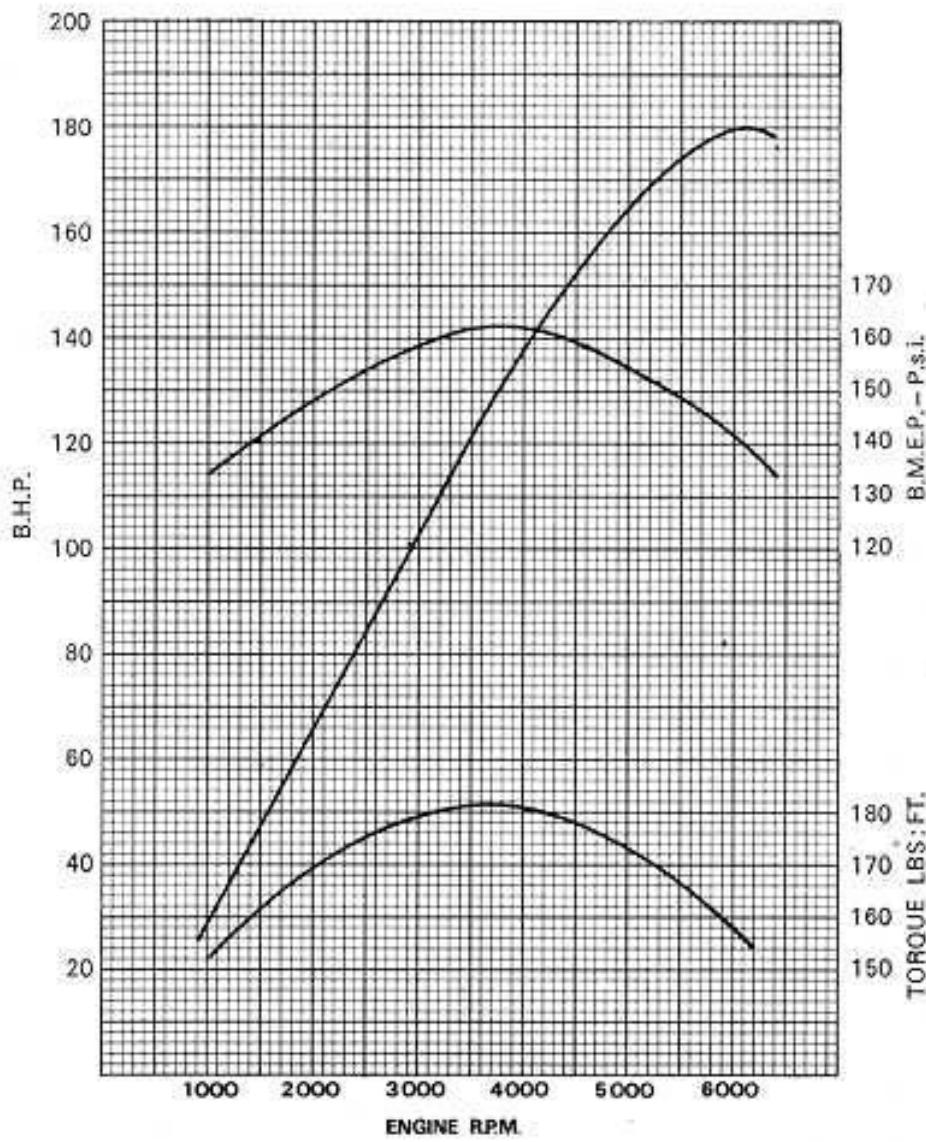
**4.2 LITRE 6 CYLINDER 92.07% BORE x 106% STROKE
