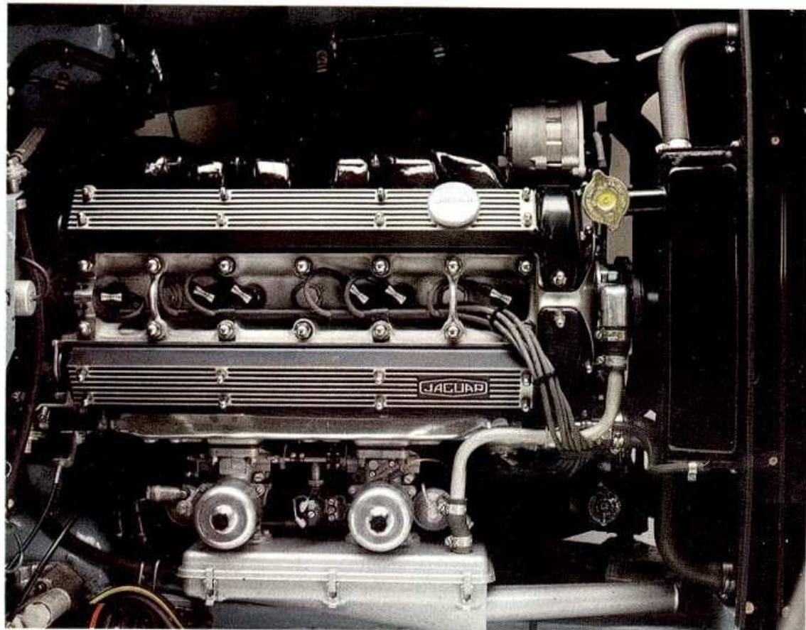
**2.8 LITRE 6 CYLINDER 83% BORE x 86% STROKE
