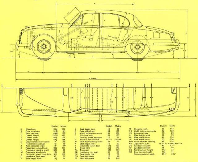
Unless otherwise stated, all dimensions are in inches and centimetres, applicable to a laden car. (Front seat shown in mid position—5" adjustment, Wheels fitted 6.40 x 15 tyres—rolling radius 12.75.)
